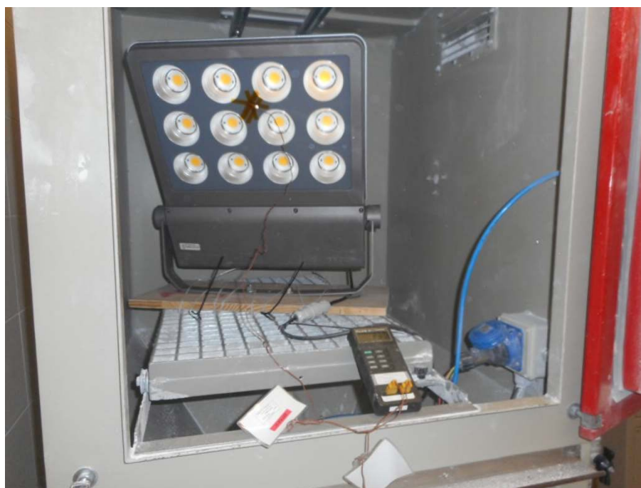
4 - Photo of test set-up – Sample 02
